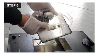
6. Press the lamp clamp and insert the new lamp. Release lamp clamp to secure lamp in place.
