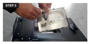
3. Once the lamp access door is removed hold the old lamp by the ceramic socket and remove the white plug from the old lamp.
