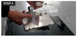
4. Press the lamp clamp to release the old lamp, and slowly remove the old lamp.
