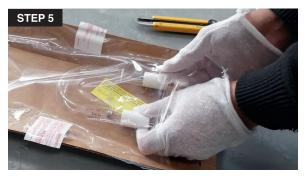
5. **Prepare the UV lamp for installation.** Remove lamp from packaging. Only after you have visually inspected the UV lamp should you break the security seal on the underside of the cardboard sleeve.
