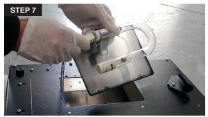
7. Holding the ceramic base, attach the plug to the new lamp. The plug will fit in one direction only. It may be necessary to rotate the plug 90° to attach it.
